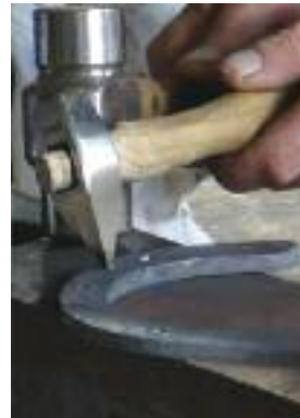
Use hammer to position forepunch to minimize heat build-up in tip. Establish your nail position and punch almost to finish depth.
